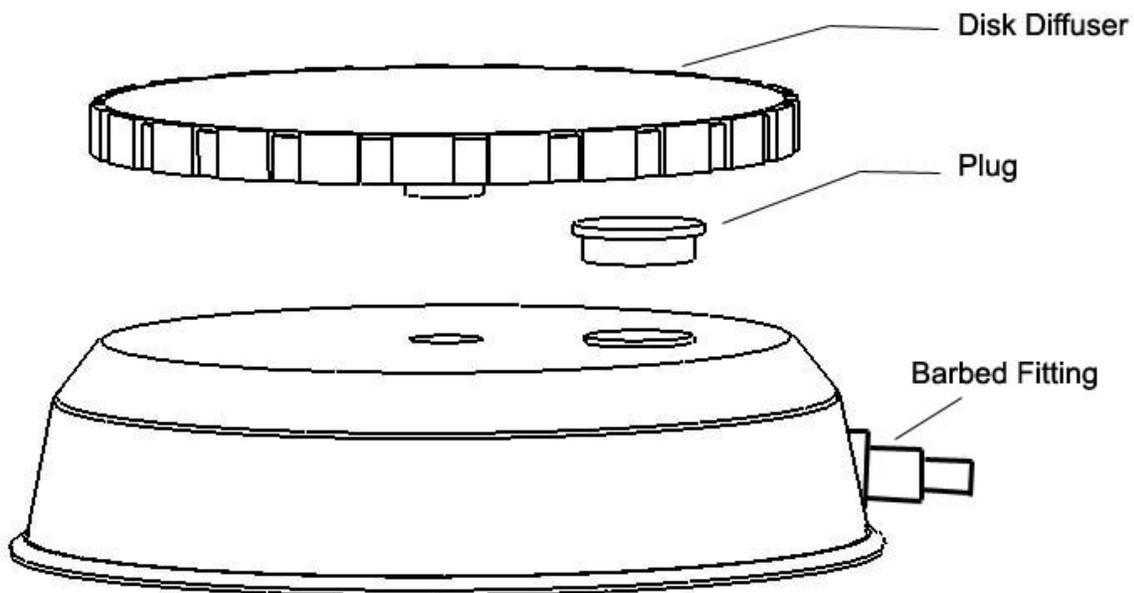
1. Fill the air station base with sand or gravel, then glue the plug using all-purpose cement. The air station base must be weighed for stability.
